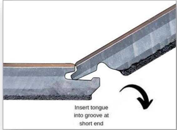
**Step 2:** Lock short end of plank by inserting tongue into groove at an angle. Then drop into place. Continue this step to the end of the row.
