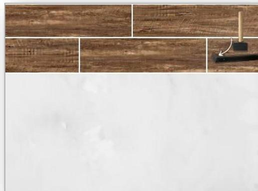
**Step 8:** Use a hammer and pull bar to lock the final piece in the row. Insert a spacer at end of the row. Continue installation on next row until final row.
