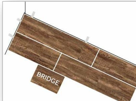
**Step 6:** Using the tongue and groove, attach a scrap piece of floor plank to bridge gap between ends of planks and hold them steady.
