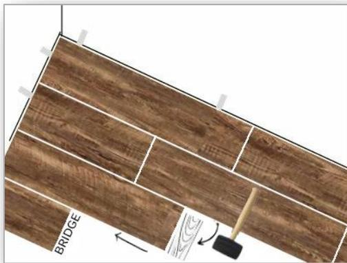
**Step 7:** Place wood block at end of plank and tap with hammer to lock ends of planks together. Remove bridge and continue toward the wall until installing the final plank in the row. BE SURE TO TAP ON EDGE OF VINYL SO AS NOT TO DAMAGE LOCKING MECHANISM OF PLANKS.
