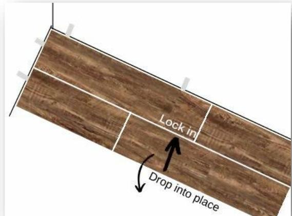
**Step 4:** Lock the long edge of plank by inserting tongue into groove at an angle and drop in place. Next, slide the plank toward the end of previously installed plank until the tongue just touches the groove.
