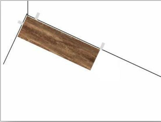
**Step 1:** Begin installation of LVP flooring from a corner of the room and working from left to right. Install spacers between the plank and the wall at the end and edges where the plank and wall come together.
