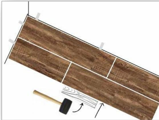
**Step 5:** THIS IS AN IMPORTANT STEP! Use a rubber mallet or hammer and a wood block. Tap the block to tap long edge of the plank to ensure a tight fit. MAKE SURE THERE IS NO GAPPING AS IT CAN COMPROMISE THE LOCKING SYSTEM!
