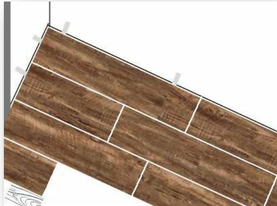
**Step 10:** To install under door jambs, use a jamb saw to undercut space under door jamb to allow the plank to slide freely. Tap the long edge with hammer and tapping block to lock in place. Use the hammer and pull bar to lock short end of plank.
