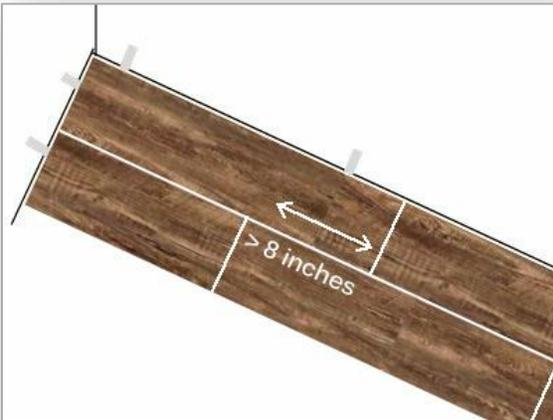
**Step 3:** Cut the last plank to fit the space. Use the leftover plank from first row as starter for second row, and so on for each row. There must be at least 8" between plank end joints on adjacent rows.\*
